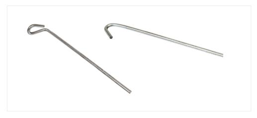
Designed to regulate the height of the ceiling metal frame. Used for suspension with a clip. It is fixed through a loop on the base reinforced concrete overlap with an anchor element.
